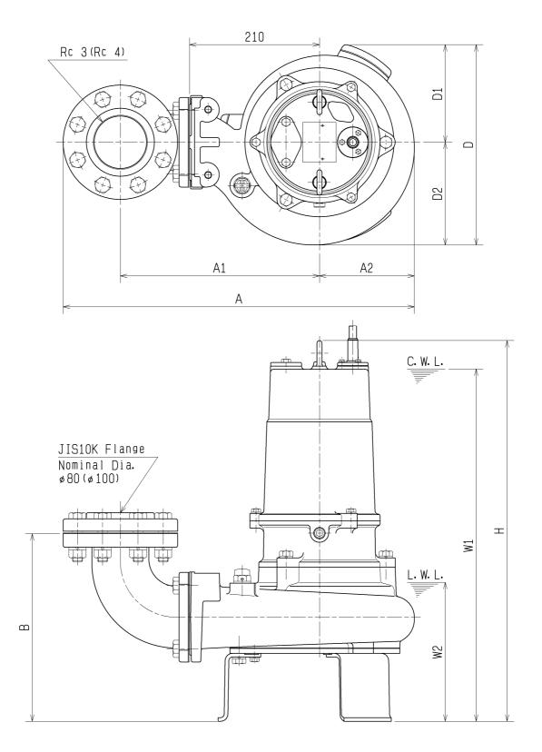
The Figure in ( ) shows the dimensions of discharge Bore at Nominal Dia  $\phi$ 100.
