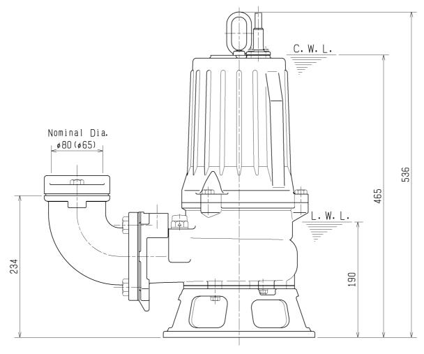
The Figure in ( ) shows the dimensions of discharge Bore at Nominal  $\phi\,65.$
