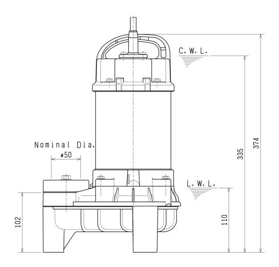
L. W. L. : Lowest running Water Level C. W. L. : Continuous running Water Level
