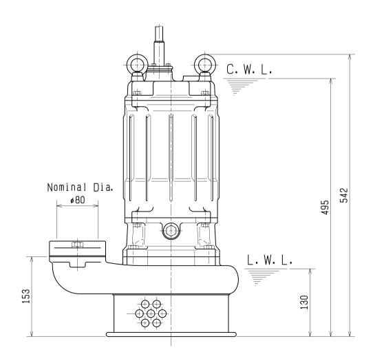
C. W. L. : Continuous Running Water Level L. W. L. : Lowest Running Water Level
