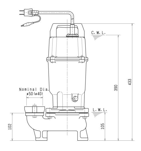
C.W.L.:Continuous running Water Level L.W.L.:Lowest running Water Level
