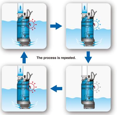
When the water level rises to contact the electric probe, pump starts operating again.
