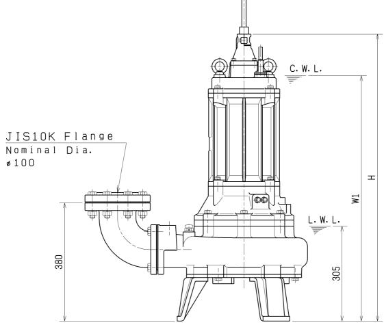
C.W.L.:Continuous running Water Level L.W.L.:Lowest running Water Level
